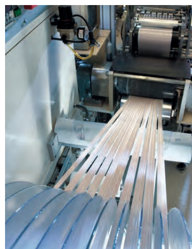
BULK FLAT FLEXIBLE CABLE PRODUCTION
